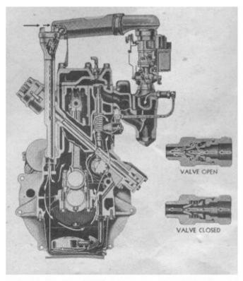
When tuning the engine of grinding valves, remove the control valve and clean it thoroughly. If this valve is blocked with carbon, the ventilating system will not operate and should the valve fail to seat, it will be impossible to make the engine idle satisfactorily.
